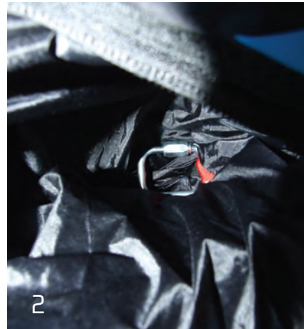
(1) "Anti-G" side pocket, (2) karabiner for attaching the drag chute bridle (3-4). Example of extracting the parachute (5-6).
