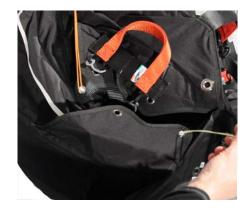
Thread a thin cord (such as paraglider riser cords) through each elastic loop. This will help close the pocket.
