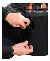
Push the metal pins on the handle into the elastic loops and under the transparent cover. It is essential to remove the cords after this operation. The cords should be pulled out slowly in order not to damage the elastic loops by excessive friction. Lastly, the handle should be positioned under the elastic cover.
