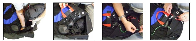
Thread a thin cord (such as paraglider riser cords) through each elastic loop. This will help close the pocket. Thread the elastic loops into the smallest of the eyelets on the pocket flaps. Close the flaps following the order shown in the photographs below.
