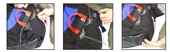
Push the metal pins on the handle into the elastic loops and under the transparent cover. It is essential to remove the cords after this operation. The cords should be pulled out slowly in order not to damage the elastic loops by excessive friction. Lastly, the handle should be positioned under the elastic cover.
