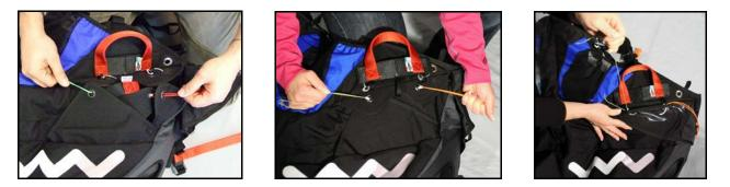
Push the metal pins on the handle into the elastic loops and under the transparent cover. It is essential to remove the cords after this operation. The cords should be pulled out slowly in order not to damage the elastic loops by excessive friction. Lastly, the handle should be positioned under the elastic cover.
